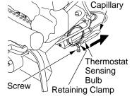
Figure 42 - Removing Thermostat Sensing Bulb
